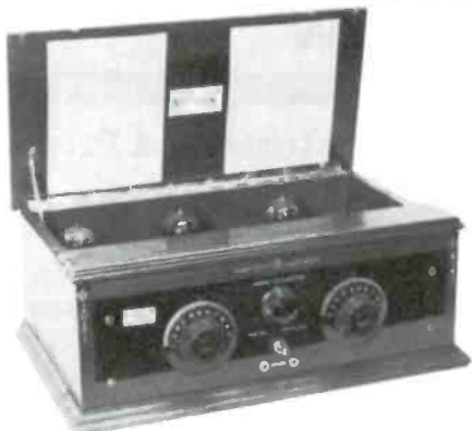
AMRAD 5-TUBE NEUTRODYNE WITH ARC-TURUS BLUE TUBES A26 AND A28 - Power input for filaments is marked 15 volts with no plus or minus signs, as these tubes accepted AC from a 15v bell transformer. This set was made circa 1923, and has regular batteries for "B". (Walter V. Worth - Wollaston, MA)
