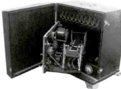
UNKNOWN BATTERY SET - The manufacturer is a mystery, but the set is too well made to be a home brew or a kit. This set uses four 199 tubes and has a built-in speaker. The panel swings out for easy access to the chassis. The antenna is inside the front door. Can anyone identify this radio? (Ron Boucher - Goffstown, NH)
