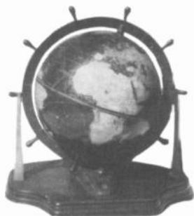
GLOBE NAVIGATOR - A novelty radio manufactured in 1939, it is tuned by rotating the world globe above. (Bob Barnes - Monroe City, MO)
