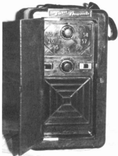
Figure 6. Plastic 1948 portable by Tom Thumb with spring-loaded front door. It was powered by AC, DC or batteries.
