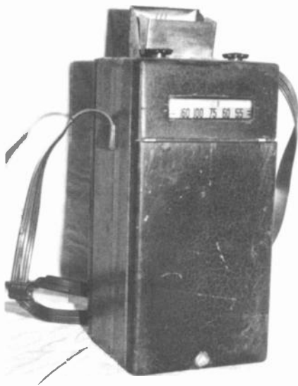
Figure 5. Rear view of Tom Thumb camera-radio which used four miniature tubes.
