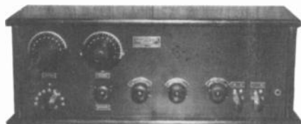
ARLINGTON RADIO - Made by the Wells Manufacturing Co. of Fond du Lac, Wisc., its circuit consists of (1) 201 RF amplifier, (1) 200 detector and (2) 201 AF amplifiers. It is a non-regenerative set and uses rather primitive AF transformers. (Donald Hatch - London, Ontario)
