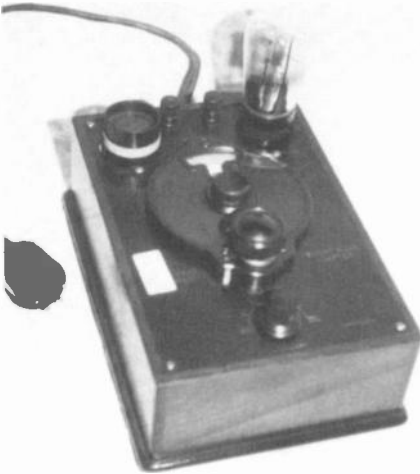
CORONADO - A battery operated radio, it was made sometime in the 1920's, I think. Tubes include 1-A-6, 30, 32, 33 and 34. (From the collection dubbed "Tony's Old Ladies.") (Anthony B. Parks - Franklin Grove, IL)
