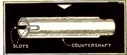
Fig. 2. Details of the connecting link between counter-shaft and crank pin. Simple and effective with enough universal joint action to take up play.
