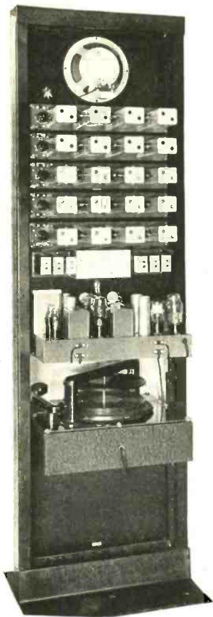
Fig. 2. Rear view of the complete high-fidelity broadcast receiver and phonograph mechanism. The speaker at the top is merely for use in tuning and adjusting.
