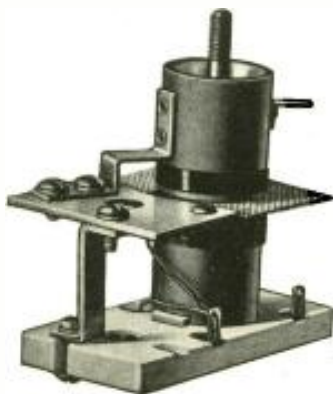
Fig. 4. One of the r-f antenna transformers with Faraday screen between windings.
