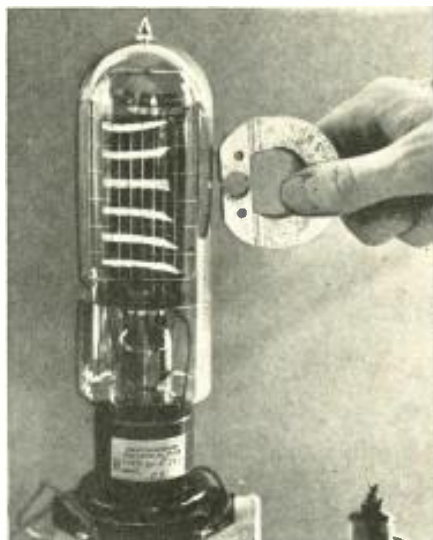
Electron pattern on plate of new tube, distorted by effects of magnet.
