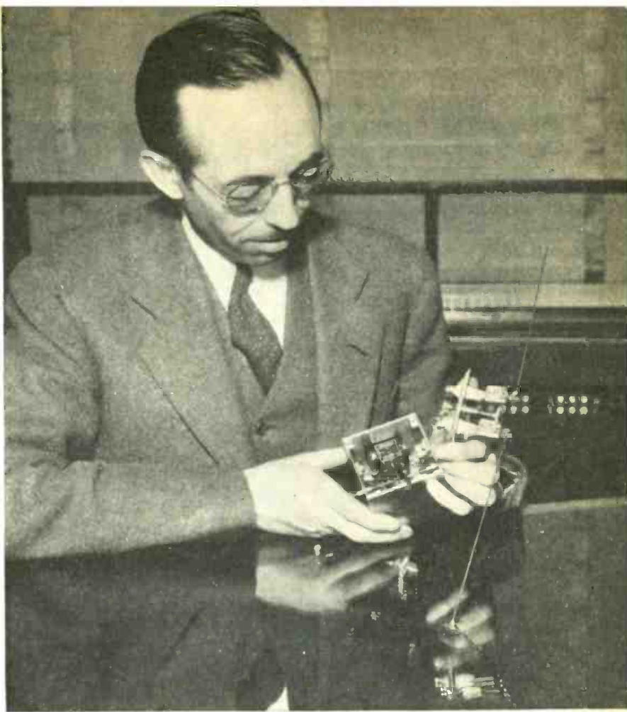
O. B. Hanson, Chief Engineer of the National Broadcasting Company, holds in his hands the world's smallest micro-wave transmitter, capable of covering a distance of four miles. The transmitter operates on wave-lengths of one meter or less. Note the "acorn tube."
