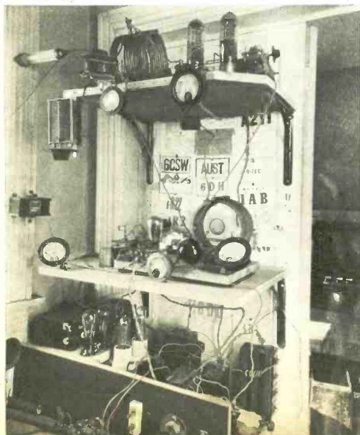
An early transmitter owned and operated by S. P. McMinn, W2WD. A pair of 211-D tubes were used. This was one of the first crystal-controlled c-w rigs.
