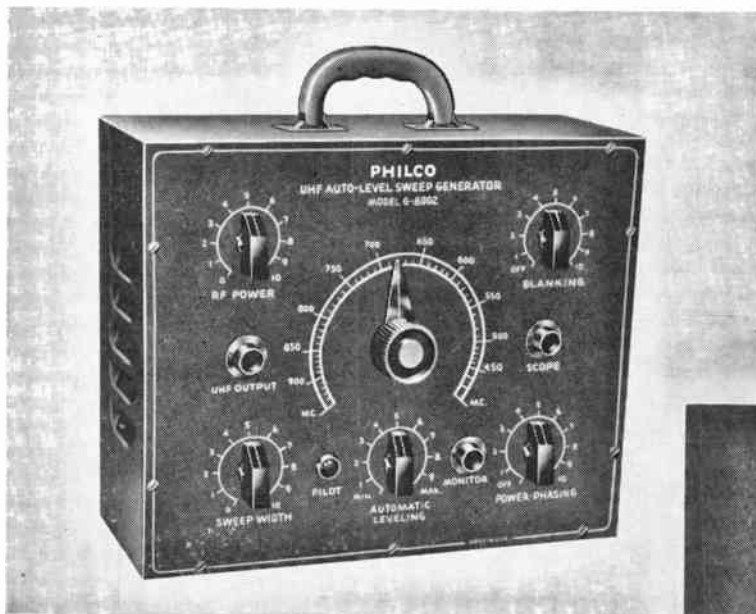
UHF Auto-Level Sweep Generator
