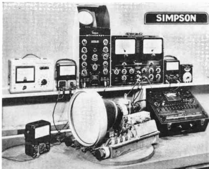
The Simpson TV-FM SiGnal Generator plus the new Simpson Mirrorscope for TV service. Simpson vacuum tube voltmeter adds volt and ohmmeter tests to the procedure.
