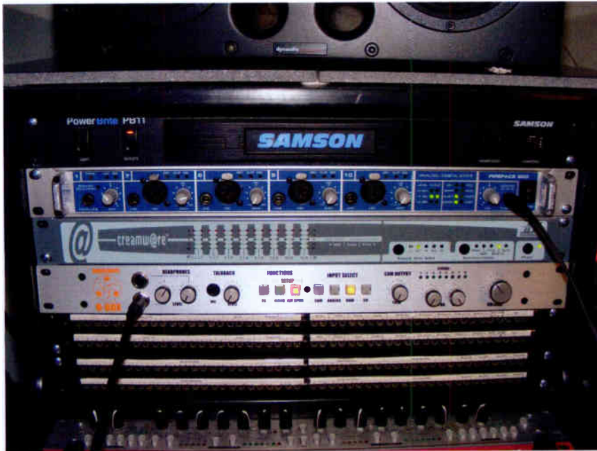
Here, an RME FireFace 800 audio interface is paired up with a Creamware A16 Ultra expander unit, to provide additional I/O.
