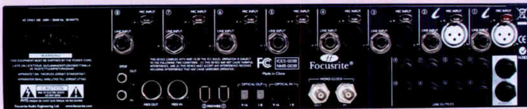
The Focusrite Liquid Saffire 56 Firewire audio interface offers several ADAT and S/PDIF digital audio ports, as well as word-clock ports.
