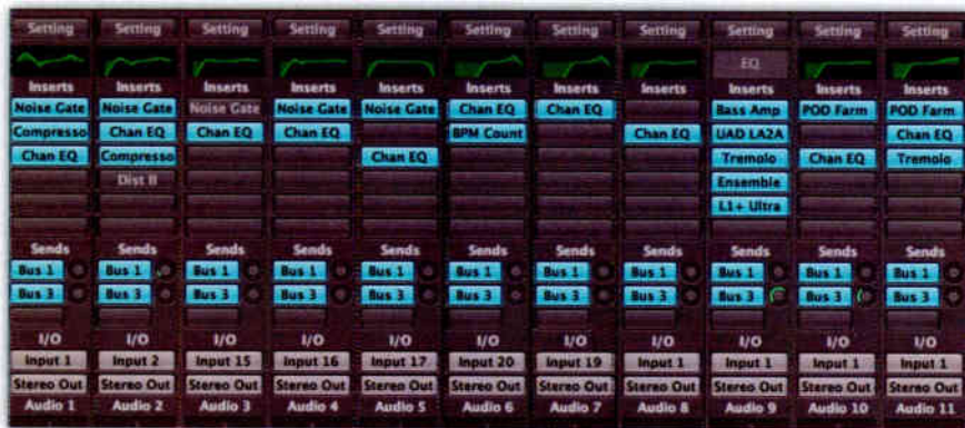
The mixer views of different DAWs will allow you to see different things. In Logic's mixer view, shown here, we can see the various different plug-ins used on each track, for example.
