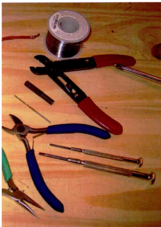
A basic wiring tool kit: soldering iron, solder, wire cutters, pliers and screwdrivers.
