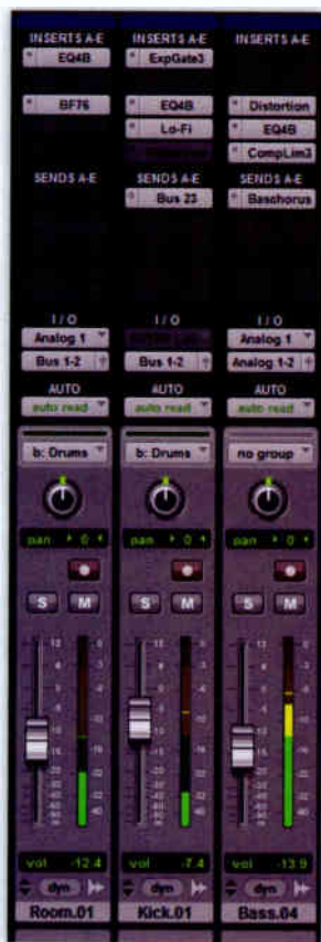
A typical view of a mixer channel strip in Pro Tools showing the inserts and sends for each channel.
