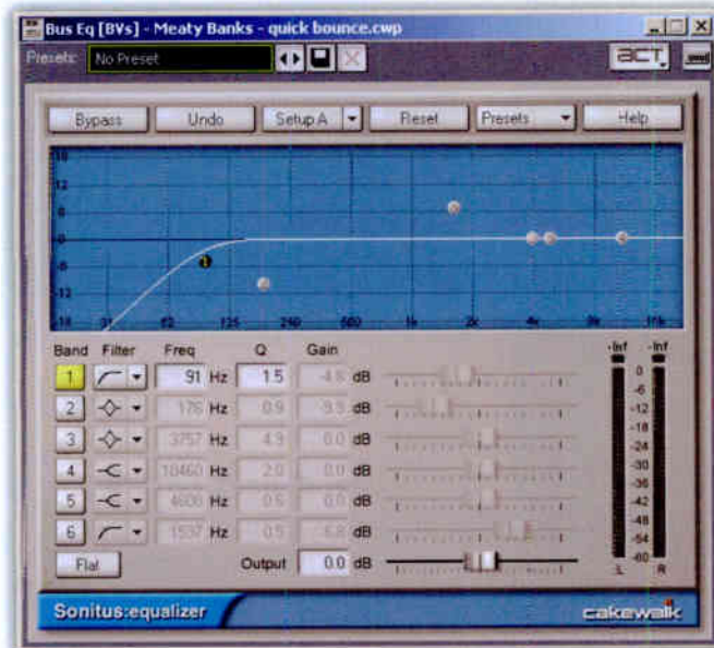
Examples of a low-cut (left) and a high-cut (right) filter from Sonar.
