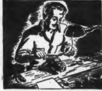
THE KEY MAKER makes the keys, hand filing them to a watch-like fit. Selmer keys are almost unbendable because the parts are Power-Hammered from cold, tough bar metal. Most instruments have cast keys.
