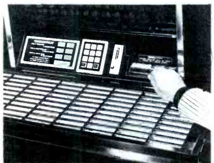
Record selection panel with ten digit buttons, bill acceptor and selection re-set buttons.
