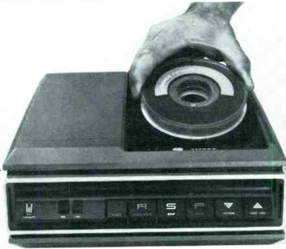
'Instavision' (left) can record & playback TV programs in color or black & white; mini-sized cartridge (center) offers 30 minutes of programming (standard) or 60 in extended play; components can be taken anywhere, like to the beach (right) where unit functions on batteries.
