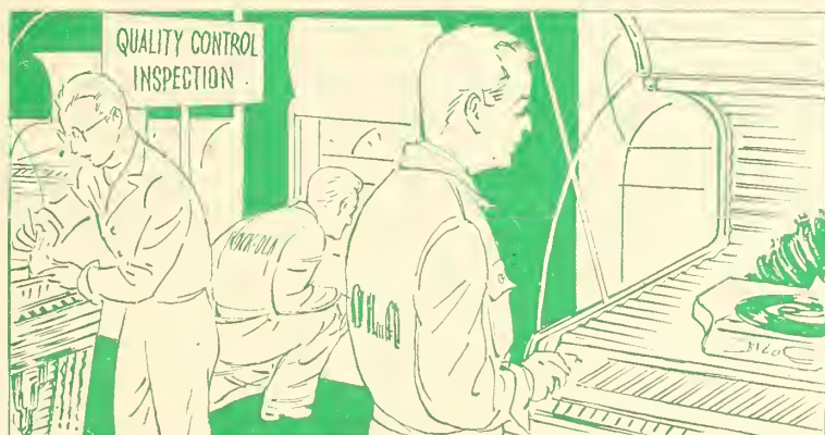
3 Every major part is then thoroughly inspected for wear, defective material and sub-standard workmanship. If it does not meet the rigid standards prescribed, it is returned to production until it does meet these requirements.
