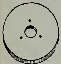
MAIN FIBRE GEAR
