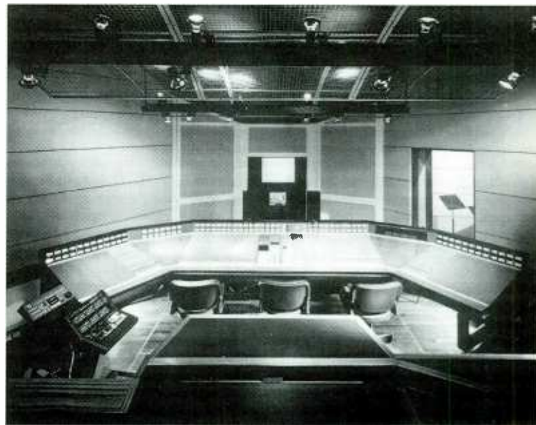
The centerpiece of Sony Music Studios' mix room A is a Solid State Logic 4096G mixing console featuring SSL's Ultimater Fader Automation System.
