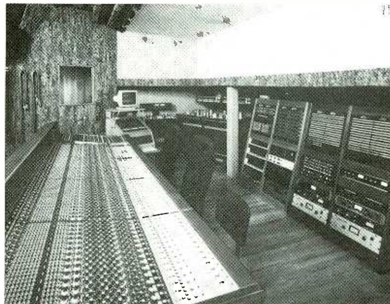
The big desk shown here is in the control room at Lighthouse Studio in North Hollywood, Calif., and is still a fairly uncommon sight in this country. The Studer 905 recording console is the first of its kind in the U.S. and was custom configured for the studio.
