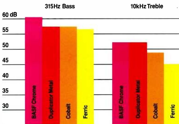
*Dynamic range is the spread between maximum output level (MOL) and noise (tape hiss). It is a major criterion of tape quality because it shows the true capacity for music. Tapes with high output and high levels of tape hiss are really no better than low output tapes with low noise. It's the difference between output and noise that matters.*
