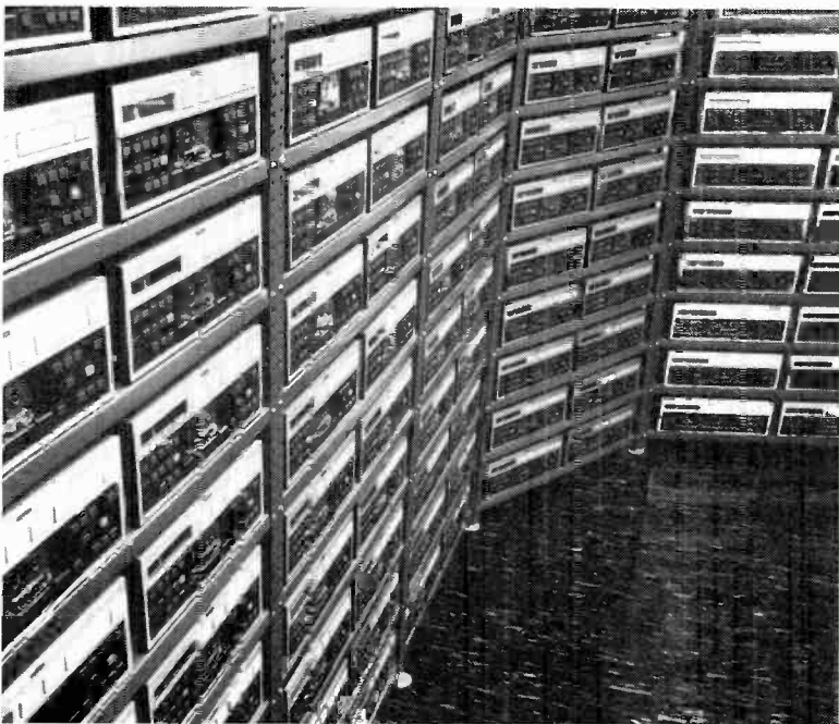
Roomful Of Revox. Some of the 200 Revox B215 consumer cassette decks recently installed at Resolution Inc., the real-time cassette duplication facility in Burlington, Vt.
