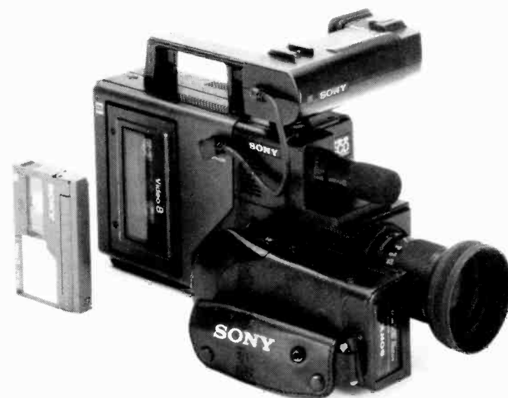
Future or Fossil? Sony Corp.'s new 8mm video camera, with 8mm videocassette, which is about the size of an audiocassette, alongside.
