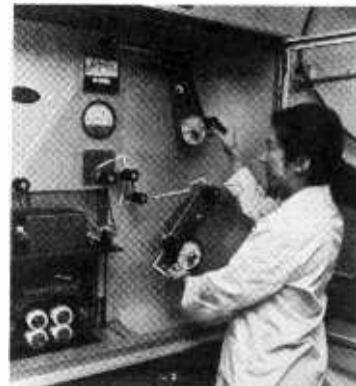
ROTARY CLEANER —A technician activates the new Peterson Full Immersion Rotary Buffer Film Cleaning machine at the facilities of Allied Film & Video, Detroit. The machine is said to revolutionize the film/video cleaning process.
