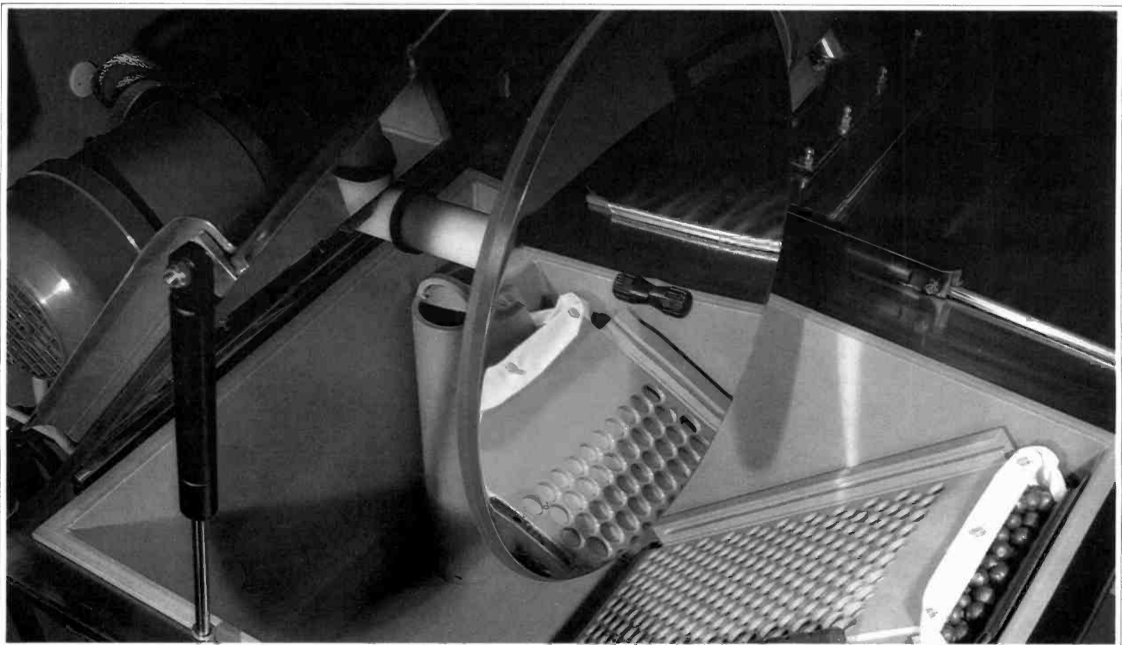
Copper Plating equipment for DMM – the result of a close German-Swedish cooperation between TELDEC and EUROPA FILM RECORD PLATING DIVISION
