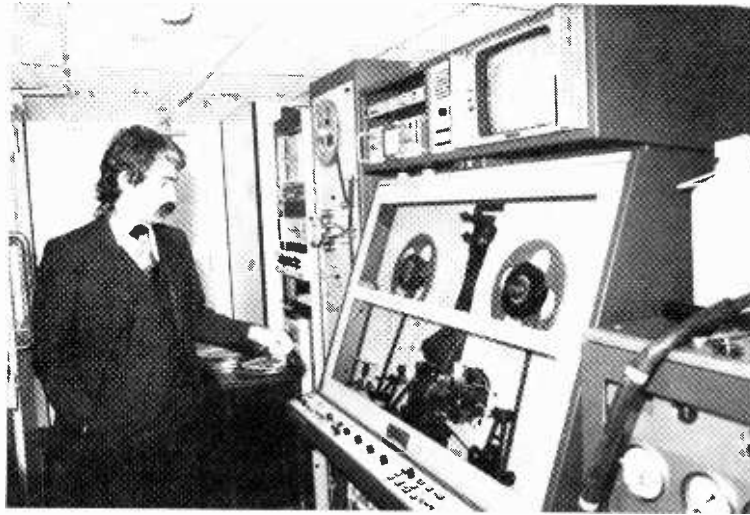
EQUIPMENT CHECK —Glen Palmer of Du Art Video examines the company's Rank color correction machine. To the right is a total-immersion liquid gate machine developed by a Hamburg engineer for use with his own Rank machine.
