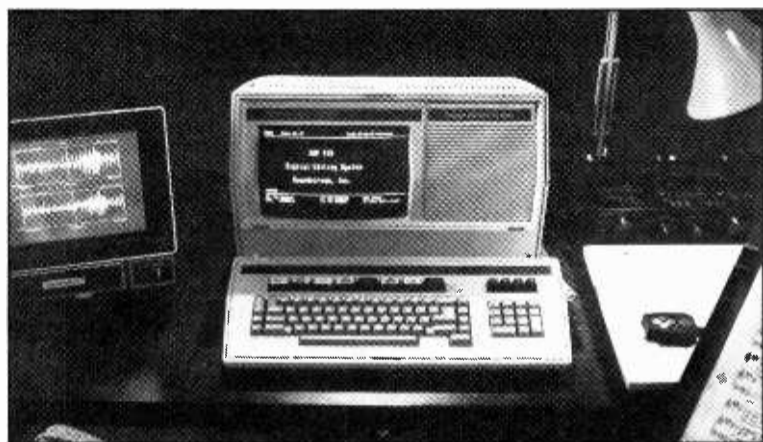
SOUNDSTREAM DIGITAL AUDIO EDITING SYSTEM: With a few keystrokes on the terminal, the producer can play any 'take' or segment of music instantly and in any order. Splices are performed by simply telling the computer what segments you want joined together and how.
