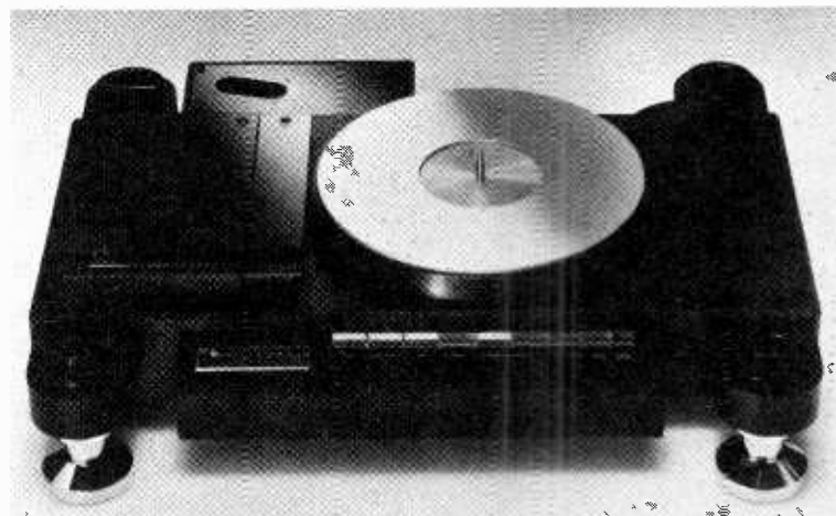
COMPUTING TURNTABLE—Nakamichi's first entry in the turntable market is the TX-1000, with a disk-drive system to automatically correct for off-centered or oversized spindle holes. A sensor arm measures the concentricity of the disk's lead-out groove and locates the record prior to playing. This model, priced at $7,000, also features accommodation for two tonearms, a direct-drive motor and PLL-servo system to provide pitch adjustment in 0.1% increments.
