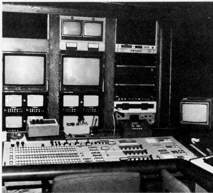
Mobile Video: A complete audio and video bus make up a formidable twin mobile recording capability for Paradise Video. Below, the inside of the video bus which features a Mach 1 editing system, Quantel effects generator, and Grass Valley switcher. Total investment: some $3 million.
