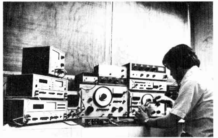
HIGH TECH AUTOSOUND —New car stereo testing facilities at Sparkomatic Milford, Pa., headquarters include an anechoic chamber, left, vibration-free and immune from sound frequencies, for accurate speaker testing, and a radio testing room, right, with double-screened walls to prevent any outside signals from entering. Equipment is designed to handle up to 35 tests. Entire six-figure investment is part of the firm's major expansion moves.
