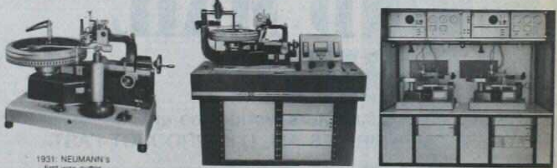
1931: NEUMANN's first wax cutter 1970: The computer controlled VMS Stereo Lathe 1974: Cutting System for the TeD Videodisk
