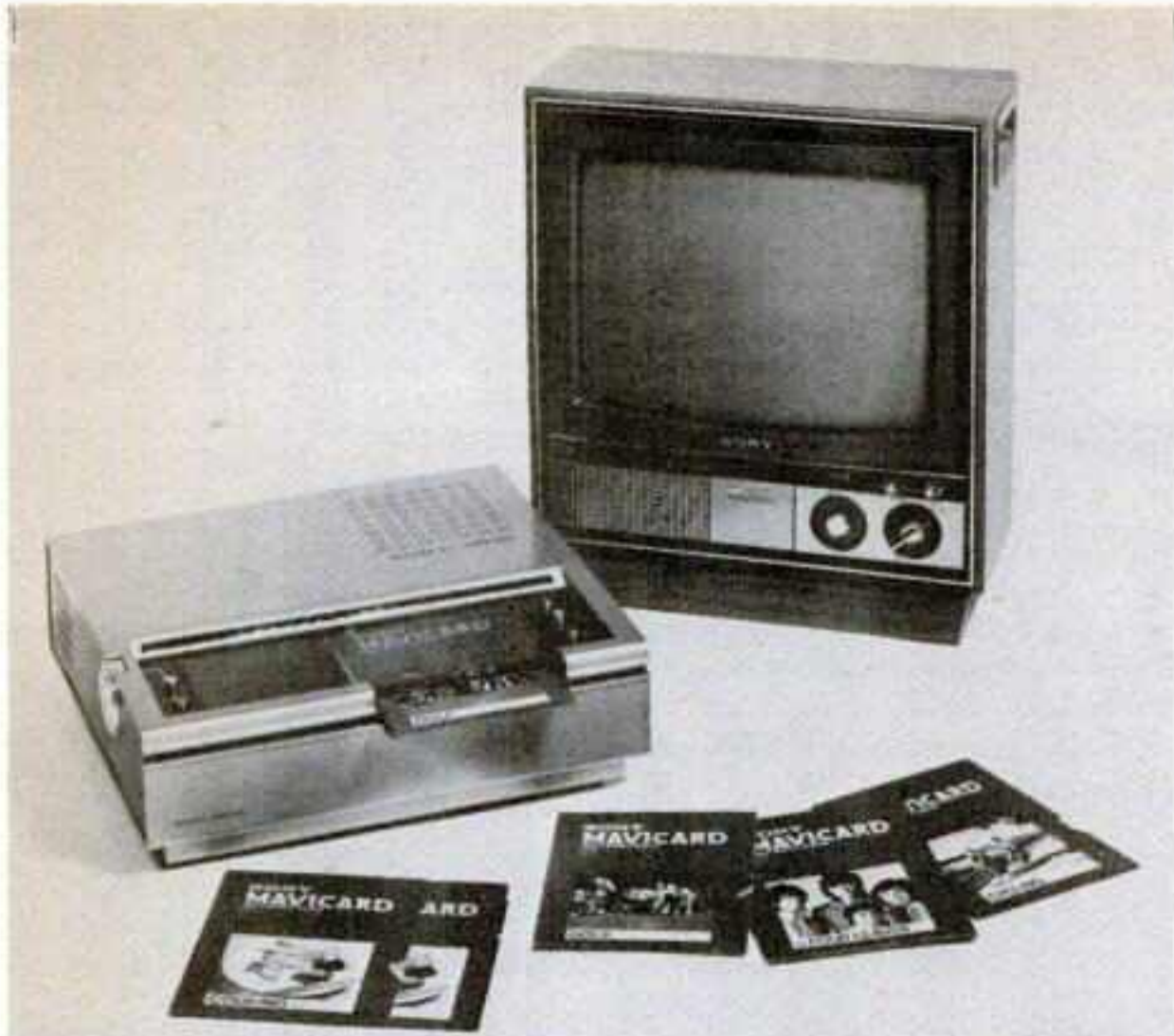
SONY MAVICA —New magnetic videotape card system recently announced (Billboard, May 25) features 6¼ x 8½-inch 10-min. Mavicards with two sheets of videotape separated after insertion in player to provide separate audio and video signals. Magnetic card is Sony answer to video disk.
