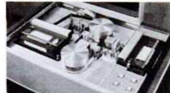
VIDEO tape contact printer developed by 3M Co. uses the S.T.A.M. method (sequential thermal anhyseretic magnetization). No mirror image master tape or recorder is necessary. The U-Matic video-cassette model operates at 37.5 ips.
