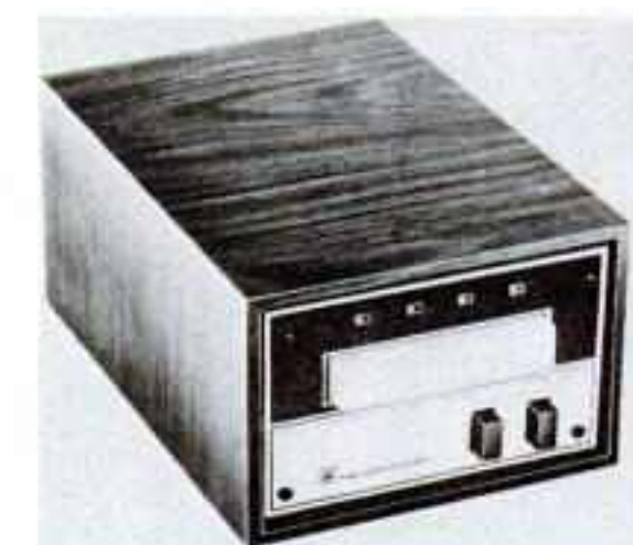
ONLY SLIGHTLY larger than the tape itself, Tenna's new Super Mini compact 8-track car stereo tape player features fine tuning, repeat function, channel indicator and slide controls. Model RR-65T lists for $69.95.
