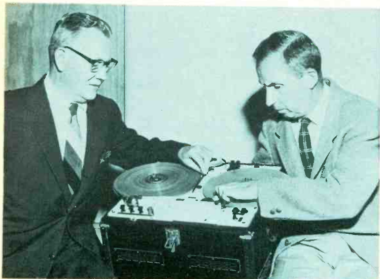
FRANK HEALY (l) and Mullin in 1947 with one of the two Magnetophons. Electronics were in a separate box.
