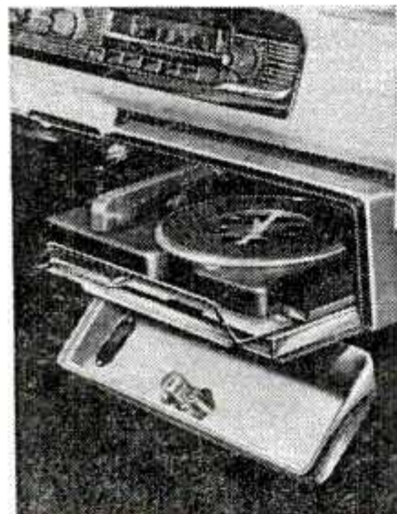
"Highway Hi-Fi" record playing unit, developed by CBS-Columbia Laboratories and featured as optional equipment with the entire line of 1956 models of Chrysler Corporation cars. Records, at 16 \frac{3}{4} r.p.m. speed, play 45 minutes of music and up to one hour of speech.
