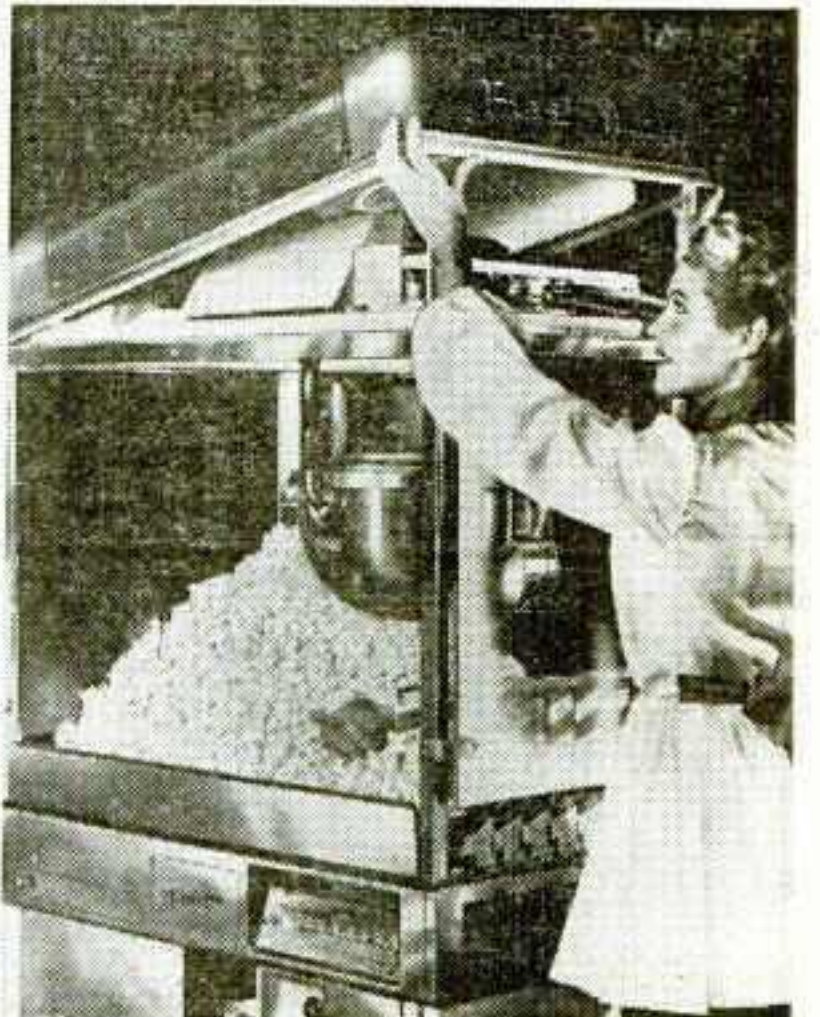
REMOVABLE HOOD permits adjustments in top of machine... Electric shock prevented by circuit breaker operating automatically as top is removed.
