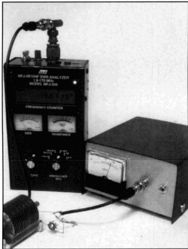
Photo A. 14-MHz L match model.
