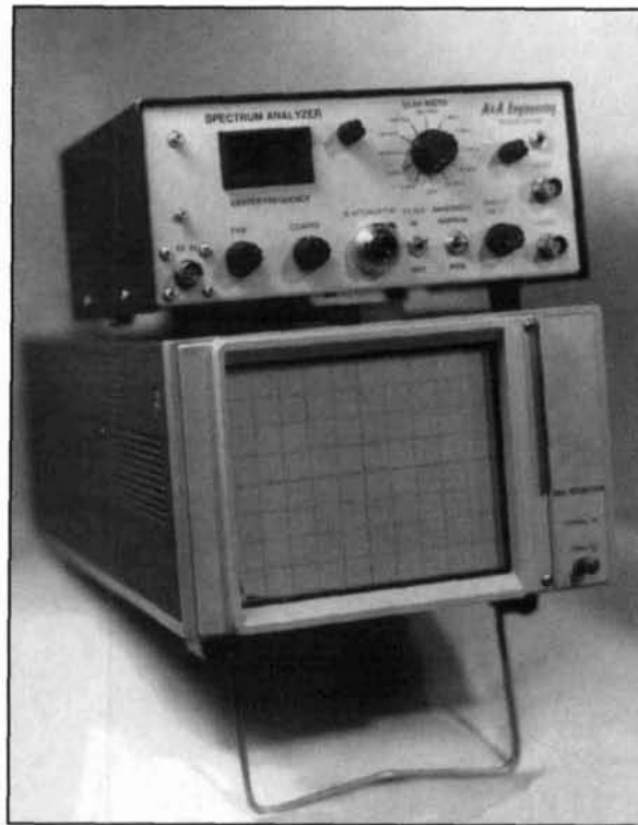
Photo A. The modified A&A Engineering spectrum analyzer and companion Tek 604 display make a dynamite combination!
