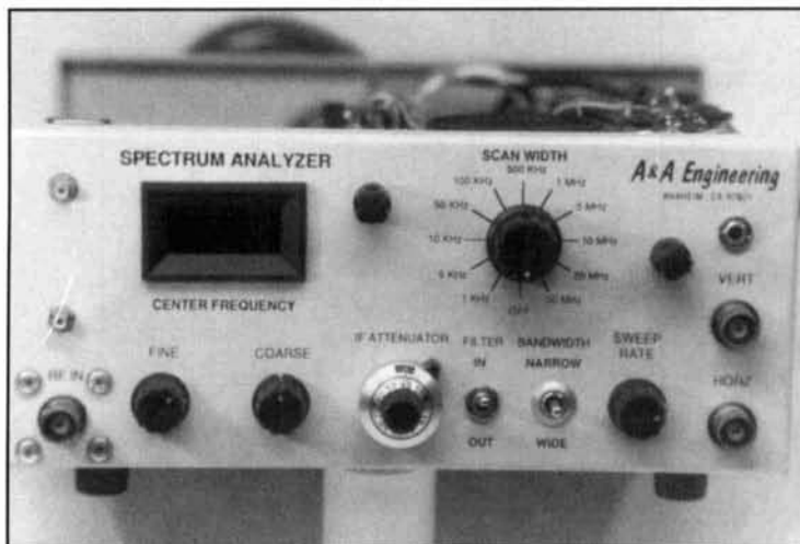
Photo D. A&A front panel after modifications. Note addition of two SMA jacks above the RF IN BNC fitting on the left. The bottom SMA supplies a calibrated -40-dBm 47.3-MHz reference signal. The upper SMA fitting is for a future tracking generator project. It supplies the divide-by-256 output from the Jerrold prescaler. To the right of the display bezel is the new IF gain control. To the right of the SCAN WIDTH control is the volume control and a jack for using an external speaker or headphones.
