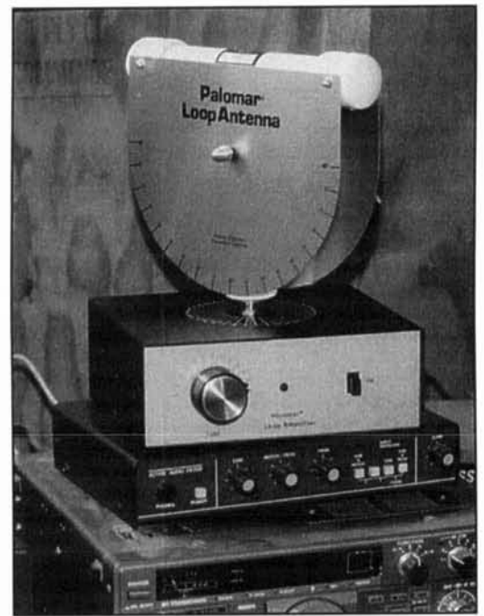
Photo F. Commercially available Palomar Engineers loop antenna. The Palomar LA-1 loop amplifier is used here and in Photo G.
