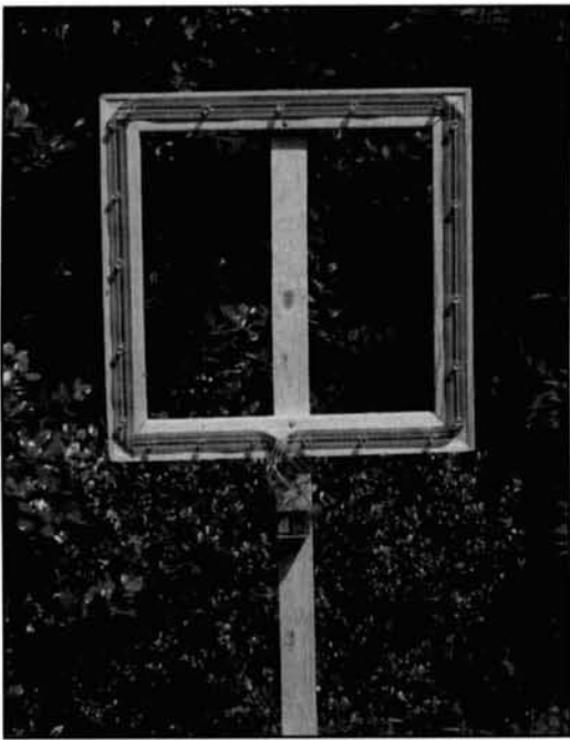
Photo D. The picture frame loop antenna.
