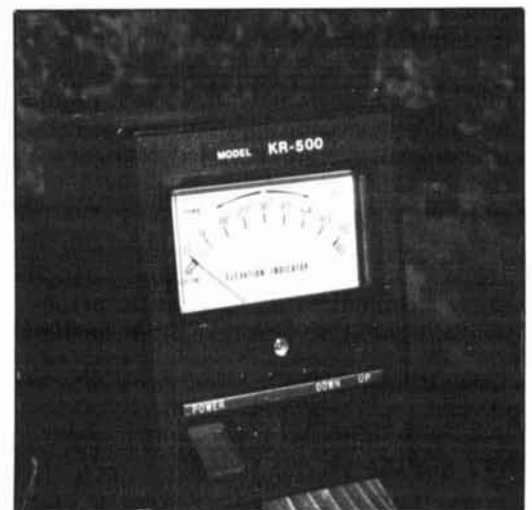
Photo C. The KR-500 control box is shown with the meter scale recalibrated in 1-degree increments. This allows easy and precise elevation readout of the array. An angle readout dial is used to set the KR-500's calibration pot to the new scale.
