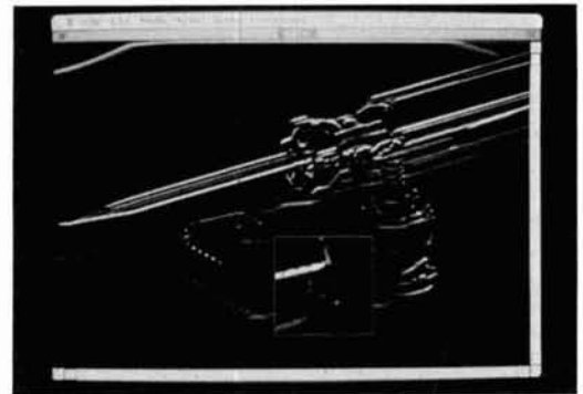
Photo F. Horizontal-edge enhancement, through convolution with a horizontal-edge enhancement kernel, attenuates all lines and edges of the original image not in the horizontal plane. Note the prominence of the EPROM body, relative to the pins, in the magnified panel.
