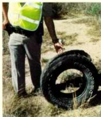
A Firestone tire from a sport utility vehicle after its tread peeled off
