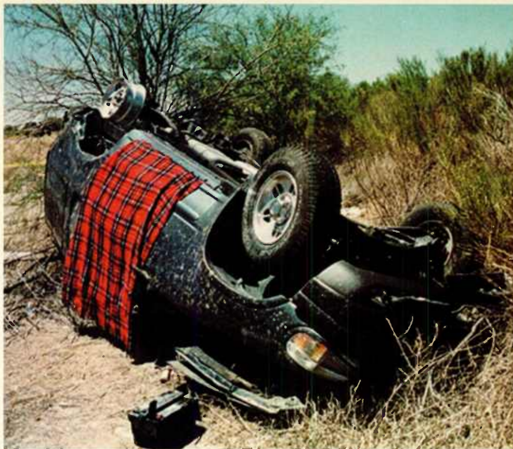
The tread separated on this Ford Explorer's left rear tire—just as Brette Lea had noticed.
