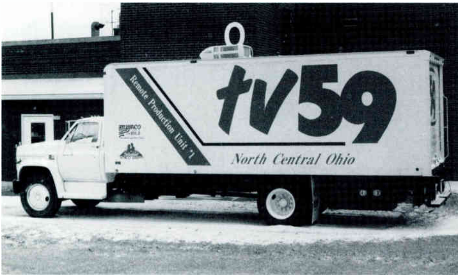
Local productions are easy with this 22-foot, three-camera production truck.
