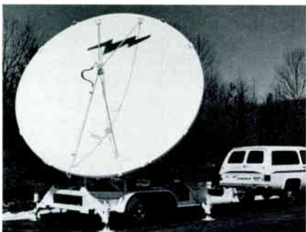
The Trifold™ 4.5 meter mobile receive/transmit ESA from Andrew.
