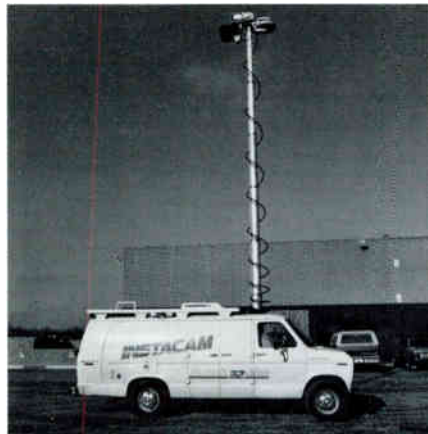
Will-Burt's Model 6-25-357/367 pneumatic telescoping mast.
