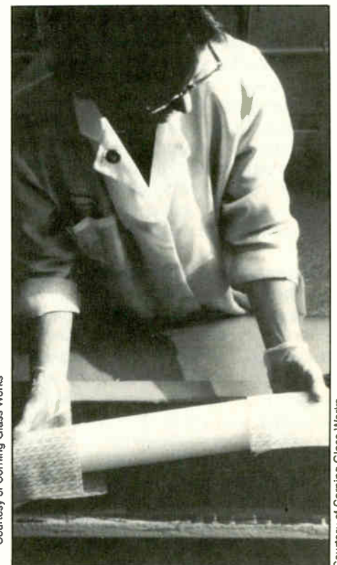
The completed preform is removed from the lathe.
