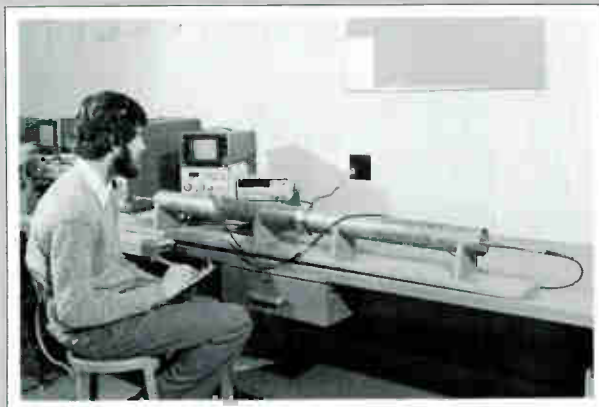
Resonant chamber for testing case leakage of Pay-TV traps (see CATJ December 1984, and September 1984 for detailed description of this apparatus).
