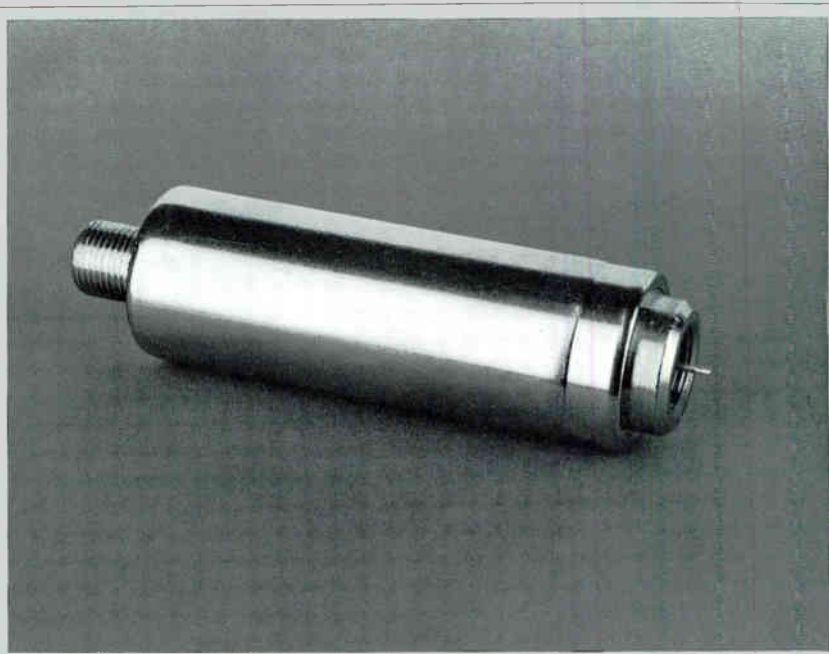
Typical cylindrical Pay-TV trap. The outer metal sleeve is forced over the end plugs which are integral with the connectors. Hence the most likely leakage source in any clearance at either end of the tube.
