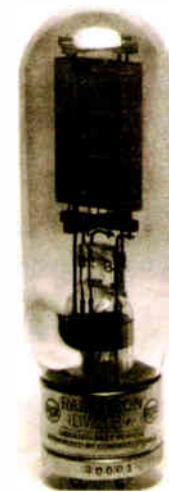
Fig. 3: A pair of Westinghouse's version (AT-21) of this very early power triode likely Heising-modulated the carrier of the “election night” transmitter.
