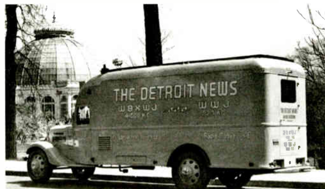
WWJ outfitted this news truck in 1938, containing the latest technology for live broadcasting and photojournalism. It contained a custom-built 100-watt shortwave transmitter and receivers. A reporter wearing a backpack transmitter could transmit back to the truck for rebroadcast to the WWJ studios via shortwave.
