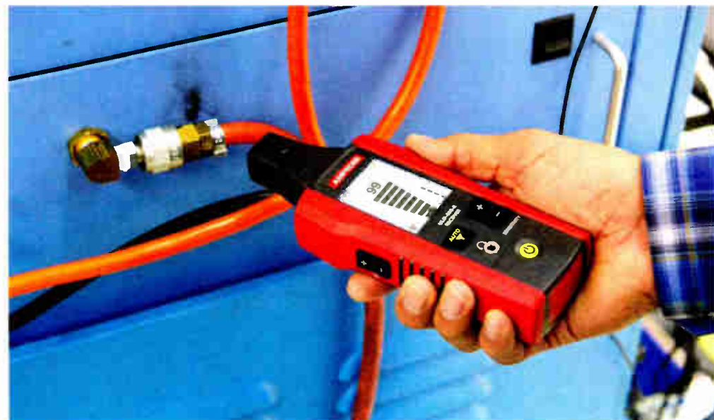
Fig. 2: Amprobe has developed an Ultrasonic Detector for leak detection.
