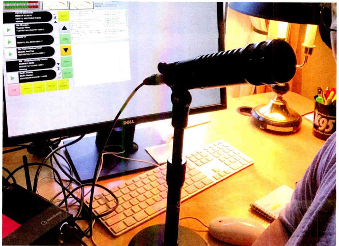
Grouped in WKHK(FM) midday host Lori Kelly's temporary COVID-19 socially distant studio are a Steinberg UR22C interface, the well-known EV RE320 microphone and WideOrbit's Distant City Voice Tracking software. It operates near a bedroom window.
