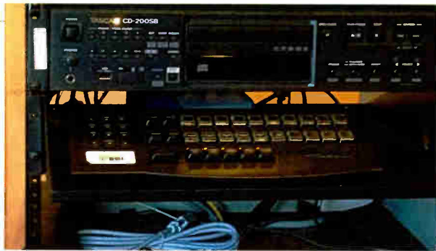
Fig 2: Reverse a rack shelf in a turret to create a shelf for a telephone controller.
