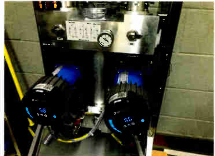
Fig. 2: The coolant pump stand showing the dual pumps.
