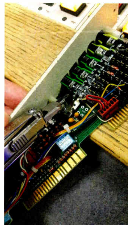
Fig. 4: Adding a tie wrap prevents the UTIL pushbutton from latching.
