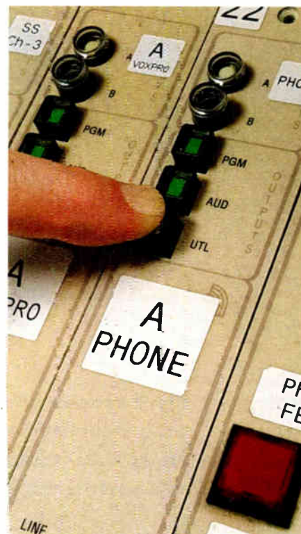
Fig. 3: In this Arrakis console, the UTIL bus is used for the mix-minus bus.
